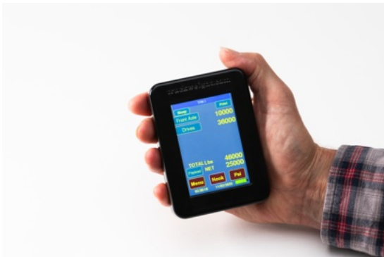
The display power cable connects to truck power 8-30 volt
