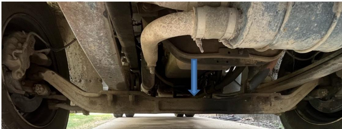
In middle on top of I-Beam, on either side of center weld seam not on top of weld seam.
