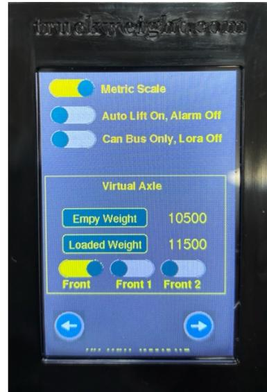
If your truck has a sensor on the front axle use this setting (Rigid truck with no fifth wheel), which turns off Virtual front axle, which is used on tractors with a fifth wheel).
