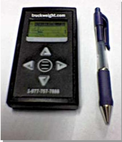
of the vehicle. Small, lightweight and durable TruckWeight is virtually worry free. It's water proof, weatherproof, shock resistant, non-corrosive and accurate in temperature extremes ranging from -40C to +70C.
