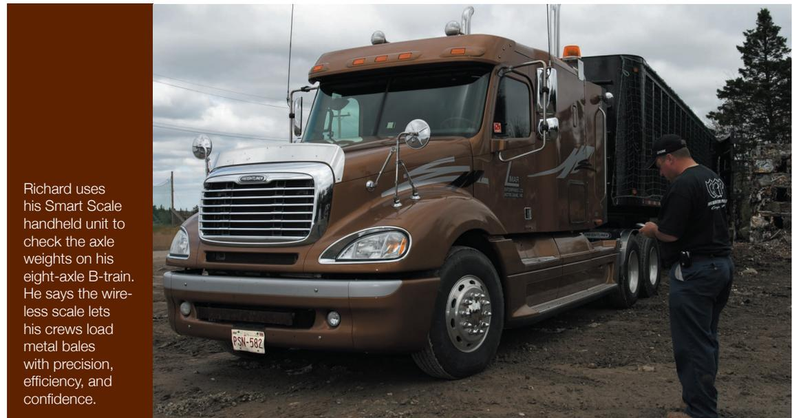
Richard uses his Smart Scale handheld unit to check the axle weights on his eight-axle B-train. He says the wireless scale lets his crews load metal bales with precision, efficiency, and confidence.
